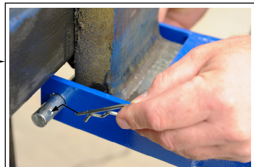
Secure tine lock pins with hitch pins
